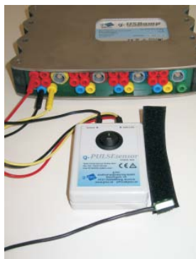
Figure 3: Pulse rate sensor with biosignal amplifier
